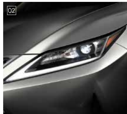
02 / Bi-Beam LED headlamps* These headlamps feature one lamp that switches between high and low beams to generate bright light for excellent visibility at night. The arrowhead-shaped DRL (Daytime Running Lamps) emit a stylish Lexus signature.
