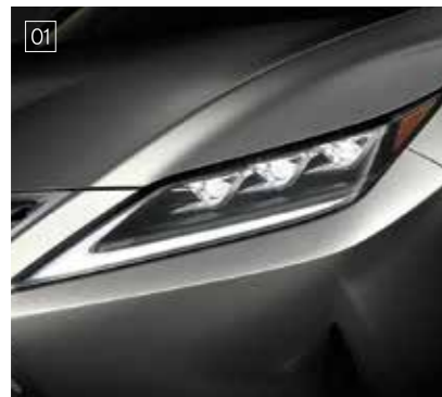
01 / The ultra-compact 3-eye bi-beam LED headlamps These ultra-compact headlamps combine a distinctive design with exceptional light distribution. The LED turn signal lamps illuminate sequentially from the inner side to the outside of the headlamps.
