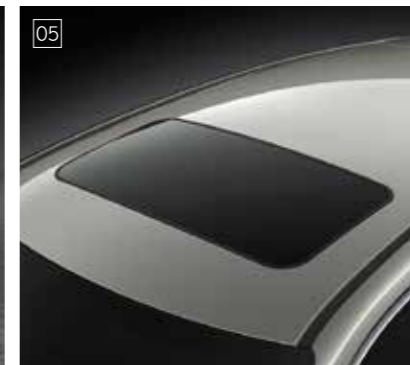
05 / Moonroof** The forward position of the moonroof enhances the feeling of openness and space in the cabin. It opens and closes, tilts up and down at the touch of a switch in the overhead console. The components were refined to reduce weight, contributing to fuel efficiency.
